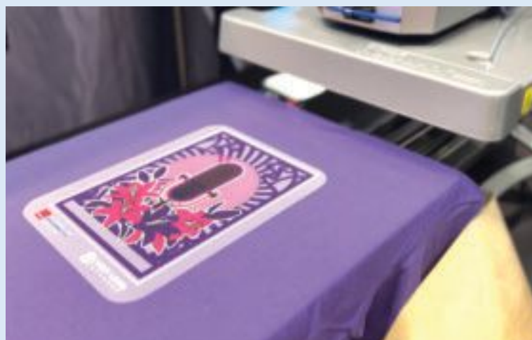
The Mimaki TxF300-75 Direct-to-Film printer finishes the white layer before transfer to a garment. Once the film is imaged, it is placed onto the garment and transferred via a heat press. | Credit: Mimaki USA
