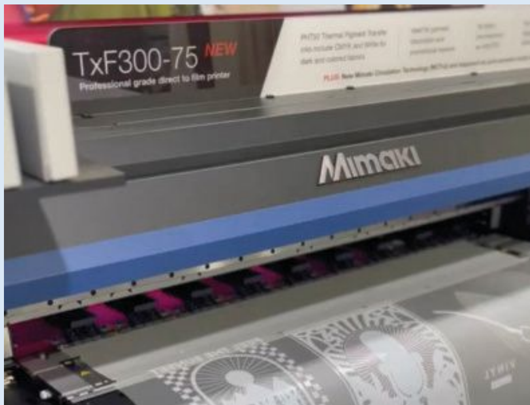
The Mimaki TxF300-75 Direct-to-Film printer finishes the white layer before transfer to a garment. Once the film is imaged, it is placed onto the garment and transferred via a heat press. | Credit: Mimaki USA
